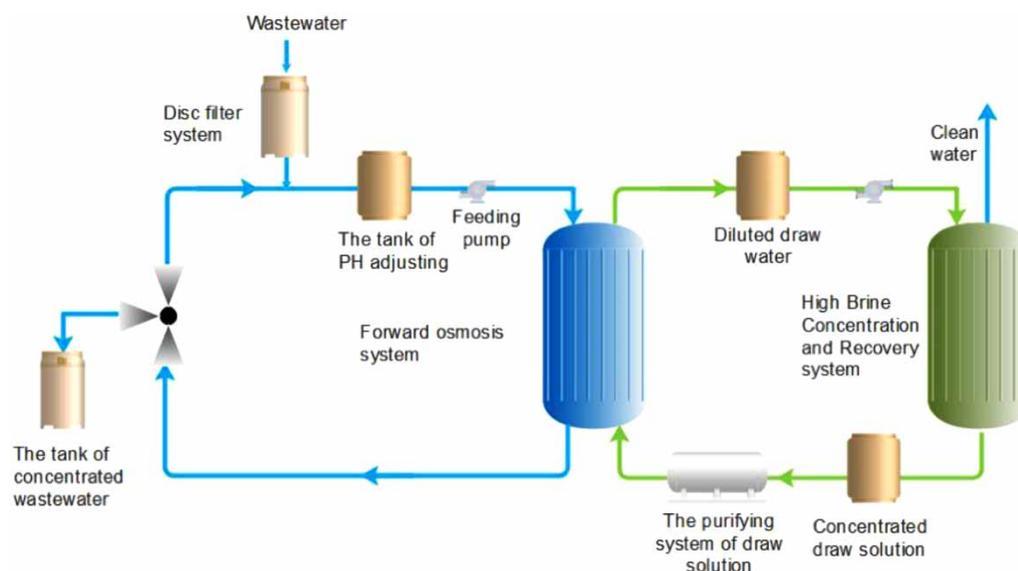
Figure 1 | Schematic representation of the OsmoBC™ treatment system.
