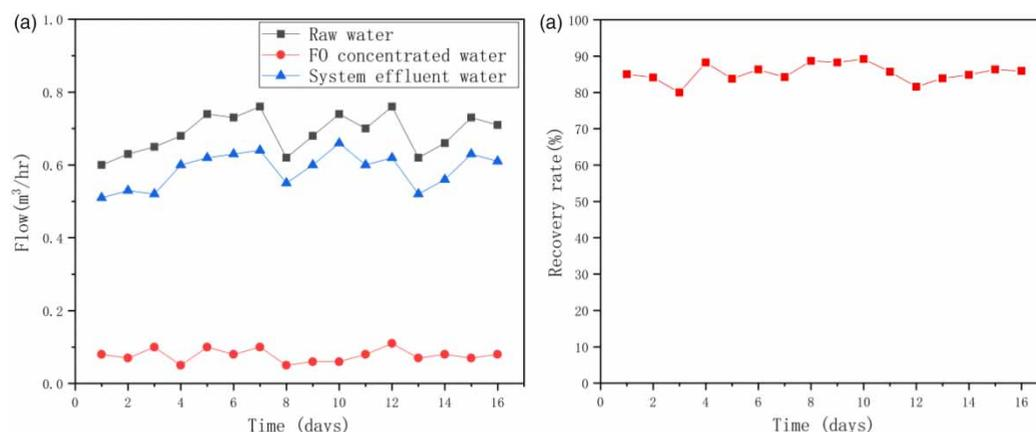
**Figure 4** | The discharge of the influent and effluent of the system (a) and the recovery rate of the system (b) with SA.
