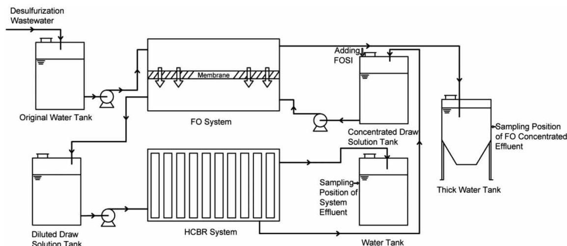
**Figure 3** | Simplified flow chart of the process of adding FO scale inhibitor.
