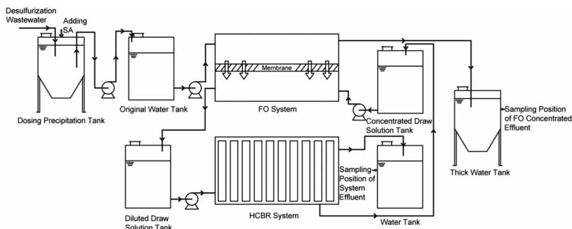
**Figure 2** | Simplified flow chart of the process of adding SA.
