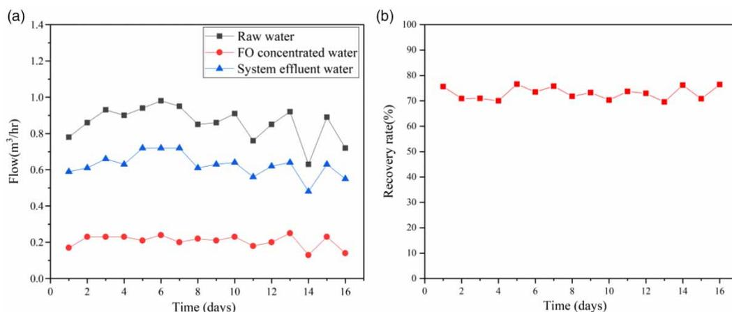
**Figure 5** | The discharge of the influent and effluent of the system (a) and the recovery rate of the system (b) with FO.
